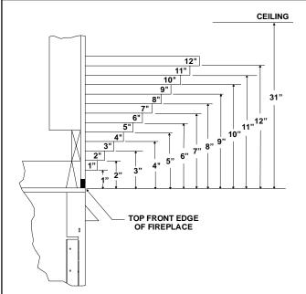
Figure 32. Minimum Vertical and Maximum Horizontal **Dimensions of Combustibles above Fireplace**
